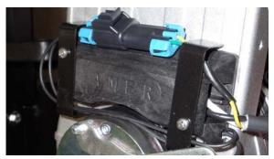
Measure the air gap distance on the brake as shown below. The air gap should measure between .012 in / .31mm and .008 in / .20mm. Take measurements from three different locations around brake. Adjust if necessary.
